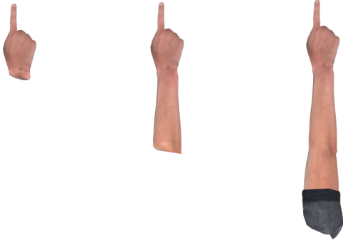
Figure 2: The virtual-arm representations: “hand only,” “hand+forearm,” and “whole arm” (from left to right). Kinect tracked the wrist and elbow joints of the participant. The virtual hand was attached to the wrist and was always aligned (parallel) to the line connecting the wrist and elbow.
